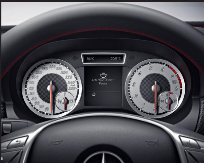
If Attention Assist calculates that the driver is flagging, it sounds a warning alarm and flashes up the symbol of a coffee cup on the dashboard
