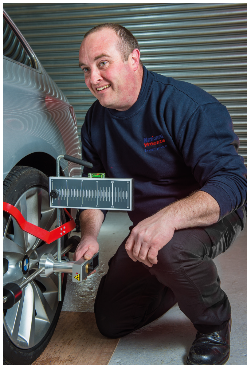
ABOVE: Aligning the CSC (Camera Sensor Calibration) tool at the rear of the car
